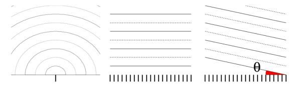
You would have to manipulate the phases of the light being emitted from the fibers. This can be done by changing the lengths of the fibers, or by changing their refractive index. For a cylinder wave to radiate away under an angle  $\theta$ , the phase at location z along the array must vary as  $\Delta \phi(z) = \frac{z}{\lambda} \tan \theta$  (with modulo  $2\pi$  as a possibility).
